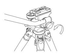
Loosen the Pan Handle Lock Knob first. Then, adjust the angle as needed and lock it.
