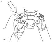
Loosen the Panning Lock Knob, and the head
