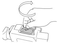
Please set the Camera Mounting Screw and the Retractable Camera Positioning Pin to holes at the camera side. Then, fix it with Mounting Wing Nut tightly.
