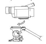
The front part of the shoe gears with the head. Please fix to make it slide into a front from the back of the head.
