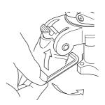
Please check the existence of slack before use. When slack is large, please adjust by the attached Allen wrench.
