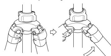
To change the angle of each leg, close the Leg slightly, and then pull the Leg Angle Adjustment Lock out.
