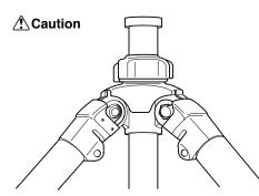
Make sure to re-attach the Base Stopper, in order to prevent the Center Column from falling out
