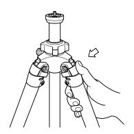
After choosing the desired leg angle, securely push in the Adjustment Lock.
