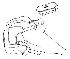
To remove the Quick Release Platform from the Pan Head, turn Quick Release Lock Lever and lift out Platform from its back.
