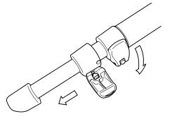
Open the Leg Lock Lever for extending/folding of tripod legs.
