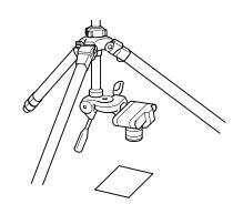
By inverting the Center Column, it is possible to do copy, and close up work.
