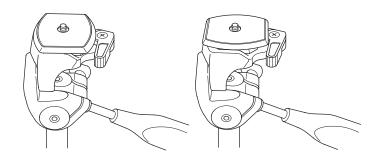
The Quick Release Platform can be attached to the camera body in either directions (along the length, or along the width).
