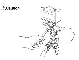
When loosening either the Pan & Tilt Handle, or the Vertical Tilt Handle, take precaution by keeping a firm grip on the handle until the Pan Head is locked down.
