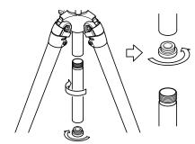
Remove the center column Base Stopper and then, remove the lower part of the center column.
