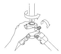
Loosen the Center Column Stopper and the Locking Collar, and then pull out the Center Column.
