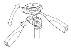
Loosen the Pan & Tilt Handle, and the head will tilt back and forth.
