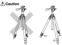
Prevent accidental equipment fall, or tripod tipping over, by making sure all levers, knobs, and handles on the tripod are securely tightened, and that all three legs are opened all the way.
