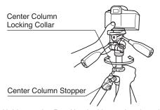
Hold onto the Pan Head with one hand, and loosen the Center Column Locking Collar with
