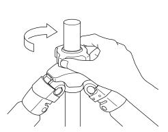
Insert the center column from lower side of main body, and tighten the locking collar and the center column stopper.
