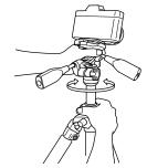
Hold onto the pan head with one hand, and loosen the center column locking collar with the other hand.
