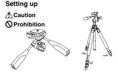
Prevent accidental equipment fall, or tripod tipping over, by making sure all levers, knobs, and handles on the tripod are securely tightened, and that all three legs are opened all the way.
