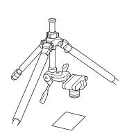
By inverting the center column, it is possible to do copy, and close up work.
