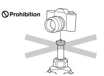
Do not attach camera directly to the threaded post of the center column.
