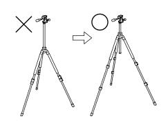
To avoid unnecessary camera vibrations, try to keep the center column height to a minimum. Also use the larger legs first, when extending
