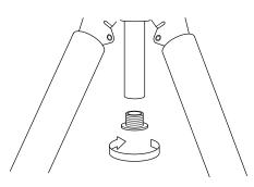
Remove the center column base stopper truning to the way arrow.
