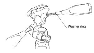
Check to see that there is a washer ring on the shaft of the vertical tilt handle, and then insert the shaft into the threaded hole located on the right side of the pan head. Screw handle all the way in until secure.
