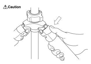
After choosing the desired leg angle, securely push in the adjustment
