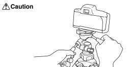
When loosening either the pan & tilt handle, or the vertical tilt handle, take precaution by keeping a firm grip on the handle until the pan head
