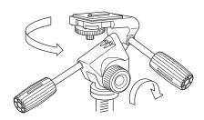
Lock the panning lock knob tightly. Grasp the pan handle and turn the whole head counter-clockwise to loosen. Then loosen the panning lock knob and it will be
