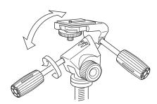
1. Loosen the panning handle to move the head freely front and rear.
