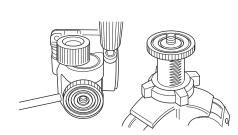
The head is installes by screwing it onto the center column's 3/8" threaded post hole.
