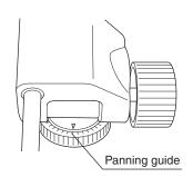
A rotating scale at the base of the head makes it easy to set exact shooting angle. To begin, set the mark at the base of the head
