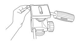
1. Both 1/4" and 3/8" camera mounting screws are supplied.
