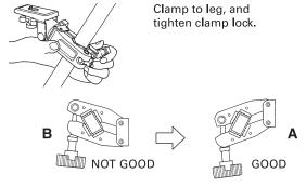
When attaching the clamp to a rectangular leg section, follow Figure A. Figure B shows the incorrect way to attach which can result in the clamp coming loose during tripod operation.
