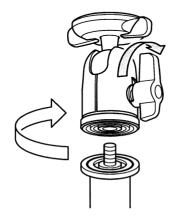
Fasten the ball locking lever and screw into a tripod mounting screw.
