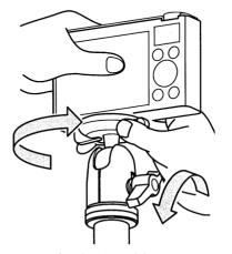
Loosen the ball locking lever. Having a camera, rotate the camera platform and fix it firmly.
