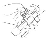
Flip up the leg lock lever to extend or shorten any of the individual leg sections to the desired length.
