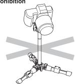
Do not set the camera towards to the between tripod legs. This setting makes the tripod unstable and may be tipping over.
