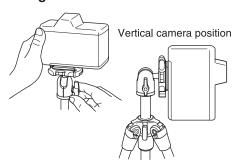
A camera can be moved freely while the ball fixing knob is loosened.
