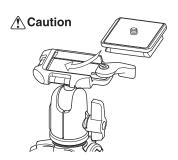
Attach the quick release shoe slid aslant from a shoe locking lever side. When it attaches, although closed automatically, a shoe locking lever is further fastened to a lever fixation-side to be fixed firmly.
