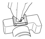
Align the length of the Platform along the base of the camera body, and securely tighten the Mounting Wing Nut.
