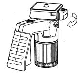
Slide into quick release shoe slantways. It will be closed automatically after attaching. Fasten the shoe locking lever tightly. It must be certainly locked.
