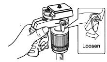
The Camera platform rotates when the Camera platform locking lever is loosened in the direction of the arrow. It moves when the Grip is grasped, and pull the Trigger. The Skirt also rotates. if the Trigger is released, it locks.
