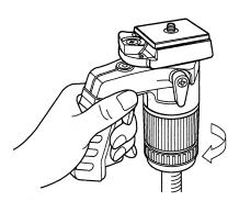
Hold Base with one hand and depress Trigger with other hand. Attach Base to center column threaded post of the tripod, and rotate it clockwise to lock in position. Release Trigger and tighten Base securely.
