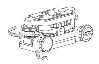
Adjust the protrusion of each plunger about 2mm, by rotating both height and azimuth pressurizing knobs. When plunger comes out from the pressurizing screw, the micro motion knobs can be operated. In case of fine adjustment range is wide, adjust both the pressurizing knob until plunger retracts.
