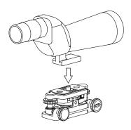
Insert wedge mounting screw to the screw to the screw hole of the field scope and rotate the wedge mounting dial until it stop.
