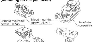
Insert pan head attachment screw of the pan head to the tripod mounting screw hole of the unit and firmly fix the unit.
