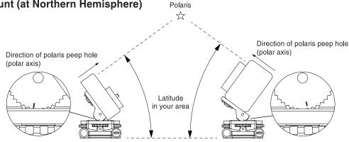
The indicator can be a good reference mark for easy and quick wedge angle setting.
