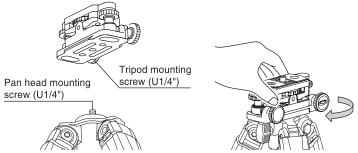
When using the unit with a field scope, attach the unit derectly to the tripod or to the pan head according to your usage.
