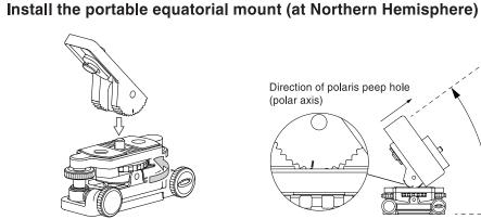
Rotate wedge mounting dial to mount the wedge to the main body.
