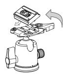
To reattach the shoe, slide it in from the shoe lock lever side.
