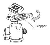
Remove the quick release shoe. Do not put the lock lever back by force as it has been stood by the stopper.
