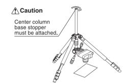
Insert the center column from the lower side of the main body, tighten the center column locking nut and the center column stopper.
