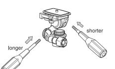
Attach the two pan handles to the pan head, by inserting the longer handle to the left, and the shorter vertical tilt handle to the right. Do not reverse.
