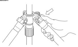
After choosing the desired leg angle, securely push the adjustment lock.
