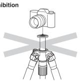
Do not attach camera directly to the attachment screw of the center column. This may damage both of camera and tripod.
