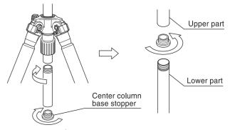
Remove the center column base stopper. Then remove the lower part of center column. Put the center column base stopper in to the upper part of center column.
