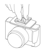
Align the length of the quick release shoe along the base of the camera body, and securely tighten the mounting wing nut.
