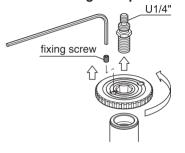
To change the U3/8" screw, loosen the fixing screw with an allen wrench (2.5mm width) and rotate the center column plate to remove from the center column. Then push put the pan head attachment screw from the bottom.
