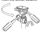
Lock the panning lock knob. Then grasp the pan or vertical tilt handle and turn the head counter-clockwise to loosen.
