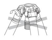
Please do not turn the center column stopper without a center column or an optional short center column attached on. The internal parts may be damaged.
