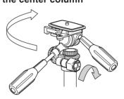
Set the pan head on the tripod's threaded post, and turn clockwise until it comes to a stop. Tighten the panning lock knob and turn clockwise slightly more.
