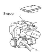
Remove the quick release shoe turning the lock lever. In this case, please do not put the lock lever back by force as it has been stood by the stopper.
