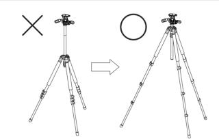
To avoid unnecessary camera vibrations, try to keep the center column height to a minimum.
