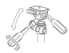
Loosen the pan & tilt handle, and the head will tilt back and forth.
