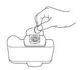
Remove the quick release shoe from the pan head turning the shoe locking lever. Do not put the shoe locking lever back by force as it has been stood by the stopper.
