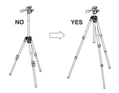
To avoid unnecessary camera vibrations, try to keep the center column height to a minimum.
