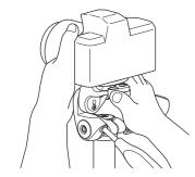
When attaching the camera to the pan head, check to make sure that the quick release shoe is engaged in the catch of the pan head before locking
