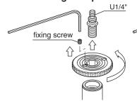
To change the U3/8" screw, loosen the fixing screw with an allen wrench (2.5mm width) and rotate the center column plate to remove from the center column. Then push out the panhead attachment screw from the bottom.
