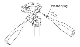
Remove the vertical tilt handle from the back of the pan & tilt handle where it is stored.
