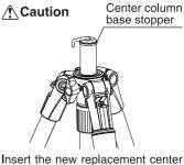
column through the top, and tighten the locking collar. Always be sure to return the center
