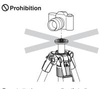
Do not attach a camera directly to the pan head
