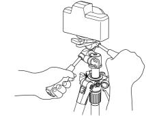
When loosening either the pan & tilt handle, or the vertical tilt handle, take precaution by keeping a firm grip on the handle until the pan head is locked down.
