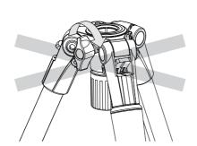
Please do not turn the center column stopper without a center column &/or an optional short center column. The internal parts may be damaged.
