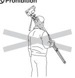
Carrying a tripod with a camera left on can result in unexpected accidents
