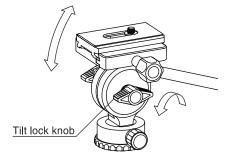
Loosen the tilt lock knob, and the head will tilt back and forth.
