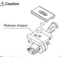
The quick release shoe can be removed from the top when the shoe lock knob is loosened fully. When the shoe lock knob is loosened fully, the release stopper mechanism does not work. Be careful not to come off the quick release shoe accidentally.
