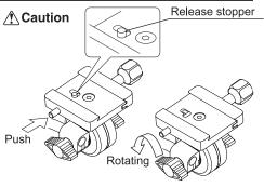
It is possible to intentionally disable the release stopper function by pressing and rotating the release lever. The release stopper is retracted into the platform. It is convenient to use a third-party quick shoe and to remove equipment. However, the stopper function doesn't work, it can cause the equipment fall.
