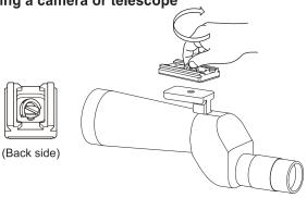
Attach the equipment screw hole and camera mounting screw and screwing lightly. Adjust the position of the quick shoe to the equipment and tighten the screw firmly.
