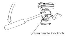
By loosen the pan handle lock knob, you can change the pan handle to the desired position. When adjusting the position of the pan handle, lock the tilt lock knob firmly.
