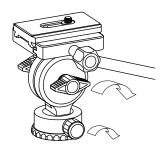
Tighten the tilt lock knob and the pan lock knob. When a pan head attachment screw of the tripod is U3/8", remove the threaded adapter.
