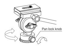
Loosen the pan lock knob, and the head will rotate along the horizontal direction.
