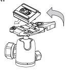
To reattach the shoe, slide it in from the shoe lock lever side.
