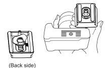
Screw the camera mounting screw on the tripod attachment screw of your camera and fix firmly.
