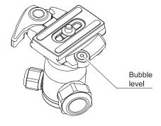
Adjust the bubble level to fit into center. The bubble level is a rough criterion. It is not accurate as a leveler on a camera.
