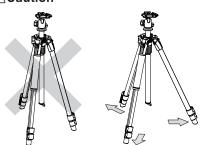
To prevent accidental equipment fall or tripod tipping over, making sure all levers, knobs and handles on the tripod are securely tightened, and all three legs are opened all the way.
