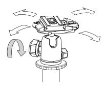
The platform can be moved freely while ball lock lever is loosened.
