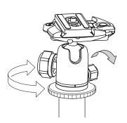
When the pan lock knob is loosened, the tripod head is rotated horizontally.
