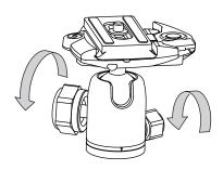
Tighten the ball lock knob and pan lock knob. When a pan head attachment screw of the tripod is U3/8", remove the double screw adaptor.
