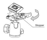
Remove the quick release shoe. Do not put the lock lever back by force as it has been stood by the stopper.
