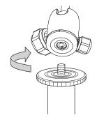
Set to the pan head attachment screw, and turn the head clockwise and fasten firmly.
