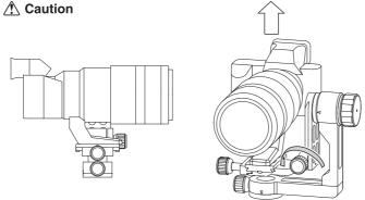
For the next step, adjust the camera height balance. Make sure shoe lock knob is securely fastened. Then, loosen the tilt lock knob and tilt the camera upwards. If the camera faces horizontal when you release the hand from the camera, loosen the vertical lock knob while supporting camera and slide the camera upwards. Please make sure the camera platform wouldn't come off from the vertical plate.
