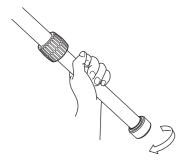
The leg tips can be converted to the spike leg tips or large rubber feet. Hold the leg pipe tightly and loosen the rubber leg tip.
