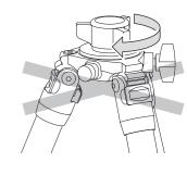
Do not rotate the center column locking collar while the center column is removed. It may damage internal parts.
