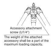
The flat base is useful when shooting in a low position or when you want to lighten the equipment. The flat base has a U1/4" screw at the bottom, and you can install some optional accessories such as the Elevator Hook 2 and
