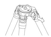
The base lock knob can be repositioned to the desired position. When the base lock knob interferes with the bottom of the camera or the head, you can pull out the lever and adjust the angle every 60 degrees.
