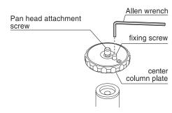
When converting pan head attachment screw of the center column from U1/4" to U3/8", loosen the fixing screw with an allen wrench (2.5mm width) and rotate the center column plate counterclockwise to remove it from the center column.
