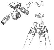
(1) Remove head from the center column before flipping the center column
