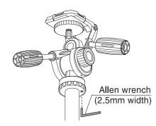
When using heavy equipment such as field scopes or telephoto lenses, use the head fixing screw to prevent the platform and tripod from loosening, use allen wrench to lock the head from the bottom of each tripod base.
