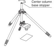
Insert the center column from the bottom of the tripod body and make sure put the center column base stopper back to the center column.
