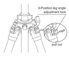
To change the angle of each leg, close the leg slightly, and then pull leg angle adjustment lock
