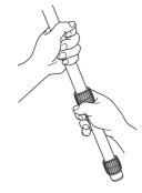
When the leg lock nut is turned to counter-clockwise, leg lock mechanism will be released and lower section of leg can be extended. Once you have pulled the leg out to the desired position, turn the leg lock nut clockwise to fix the leg.
