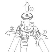
When replacing the base, 1 Loosen the base lock knob
