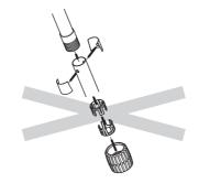
Do not remove the leg lock nut and inner parts. It will cause tripod malfunction or result in missing parts. In case the leg unit is disassembled, please refer to the figure below to reassemble the parts correctly.
