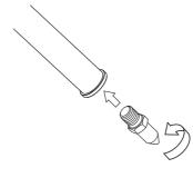
Screw the spike leg tip into the leg pipe until it comes stop. Then the spike leg tip must be further tightened with the included wrench. Always use the attached wrench for replacement to avoid pipe damage.
