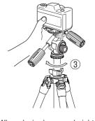
3 When desired camera height is acquired, twist the center column locking collar clockwise and lock the center column.
