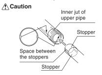
Match the space between two stoppers and inner jut of upper pipe when the pipe is inserted.
