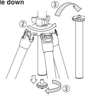
(2) Loose the center column locking collar (3) Remove the center column base stopper, and pull out the center
