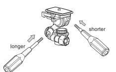
Attach the two pan handles to the pan head, by inserting the longer handle to the left, and the shorter vertical tilt handle to the right.
