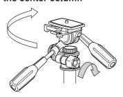
Set the pan head on the tripod's threaded post, and turn clockwise until it comes to a stop.
