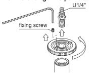
To change the U3/8" screw, loosen the fixing screw with an allen wrench (2.5mm width) and rotate the center column plate to remove from the center column. Then push put the pan head attachment screw from the bottom.
