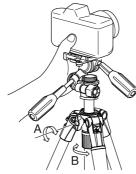
Center column stopper is used to lock or unlock center column.
