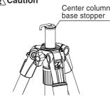
Insert the center column from the lower side of main body, and tighten the center column locking nut and the center column stopper.
