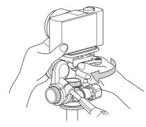
When you fix this quick release shoe to pan head, the quick release lock lever will return to the original position automatically.
