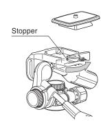
Remove the quick release shoe turning the lock lever. In this case, please do not put the lock lever back by force as it has been stood by the stopper.
