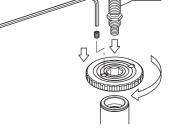
Flip the pan head attachment screw and put back to the center column plate. Screw in the center column plate and the pan head attachment screw. Tighten the fixing screw to avoid the rotating the center column plate while in use.
