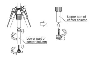
Remove the center column base stopper and then, remove the lower part
