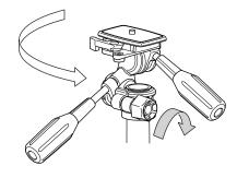
First, lock the panning lock knob, then grasp the pan, or vertical tilt handle and turn the head, counter-clockwise to loosen.
