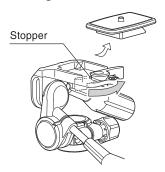
Remove the quick release shoe turning the shoe locking lever. In this case, please do not put the shoe locking lever back by force as it has been stood by the stopper.
