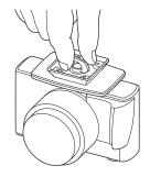
Align the length of the quick release shoe along the base of the camera body, and securely tighten the mounting wing nut.
