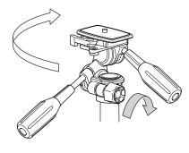
Set the head on the tripod's threaded post, and turn clockwise until it comes to a stop. Tighten the panning lock knob and turn clockwise slightly more.
