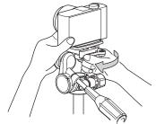
When you fix this quick release shoe to pan head, the shoe locking lever will return to the original position automatically.
