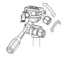
Loosen the vertical tilt knob or vertical tilt handle, and the level can be adjusted.
