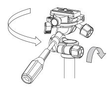
First, lock the panning lock knob, then grasp the pan, or vertical tilt handle and turn the head, counter-clockwise to loosen.
