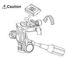
Fix the shoe lock knob firmly after inserting the quick release shoe to the platform. Please make sure the equipment is securely fixed to the pan head, before you use the pan head.
