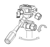
Loosen the panning lock knob, and the head will rotate horizontally.
