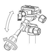
Loosen the pan & tilt handle, and the head will tilt back and forth.
