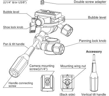
\*Bubble level is a rough criterion. It is not accurate as a leveler on a camera.
