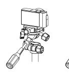
For conventional use, the platform faces sideways, and the front is for using a field scope or telephoto lense that requires fore-aft COG adjustment.
