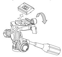
Remove the quick release shoe to loosen the shoe lock knob until the quick release shoe can be removed from the platform.
