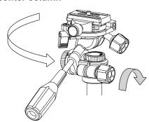
First, lock the panning lock knob, then grasp the pan, or vertical tilt handle and turn the head, counter-clockwise to loosen.
