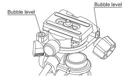
Adjust the level so that the bubble in inside of the marked circle.
