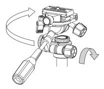
Set the head on the tripod's threaded post, and turn clockwise until it comes to a stop. Tighten the panning lock knob and turn clockwise slightly more.
