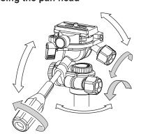
Loosen the pan & tilt handle, and the head will tilt back and forth.
