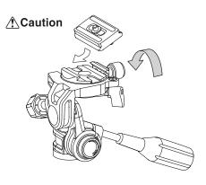
Fix the shoe lock knob firmly after inserting the quick release shoe to the platform.
