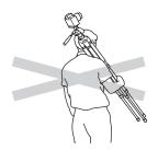
Carrying a tripod with a camera left on can result in unexpected accidents
