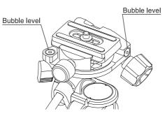
Adjust the level so that the bubble in inside of the marked circle.
