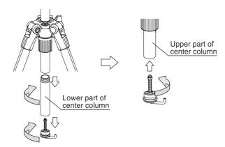
Remove the center column base stopper and then, remove the lower part of center column.
