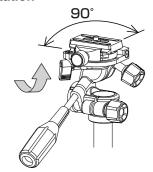
The platform rotates 90° when the platform lock knob is loosened. Once the camera is in place, fasten the platform lock knob.
