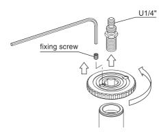
To change the U3/8" screw, loosen the fixing screw with an allen wrench (2.5mm width) and rotate the center column plate to remove from the center column
