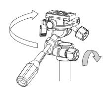
Set the head on the tripod's threaded post, and turn clockwise until it comes to a stop.
