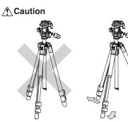
To prevent accidental equipment fall or tripod tipping over, making sure all levers, knobs and handles on the tripod are securely tightened. And all of the three legs are opened completely.
