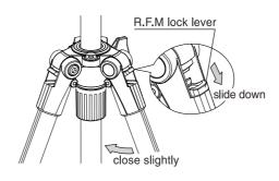
Close the leg slightly and slide the R.F.M lock lever
