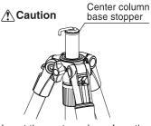
Insert the center column from the bottom of main body, and tighten the center column locking nut and the center column stopper.
