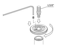
Flip the pan head attachment screw and put back to the center column plate. Screw in the center column plate and the pan head attachment screw. Tighten the fixing screw to avoid rotating the center column plate while in use.
