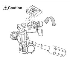
Fix the shoe lock knob firmly after inserting the quick release shoe to the platform.
