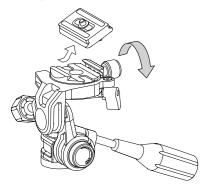
Remove the guick release shoe to loosen the shoe lock knob until the quick release shoe can be removed from the platform.
