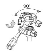
The platform rotates 90° when the platform lock knob is loosened.
