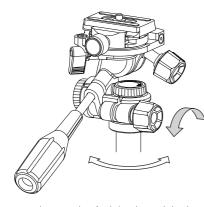
Loosen the panning lock knob, and the head will rotate horizontally.
