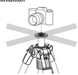
Do not attach a camera directly to the pan head attachment screw of the center column. This may damage both your camera and tripod.
