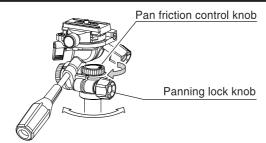
While loosening the pan & tilt handle, simultaneously tighten the tilt friction control knob until vertical movement becomes stiff. While loosening the panning lock knob, simultaneously tighten the pan friction control knob until horizontal movement becomes stiff. If the pan handle is too loose, it won't allow smooth movement.
