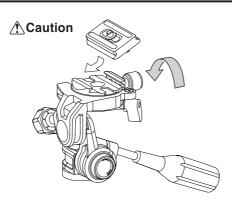
Fix the shoe lock knob firmly after inserting the quick release shoe to the platform. Please make sure the equipment is securely fixed to the pan head, before you use the pan
