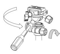
First, lock the panning lock knob, then grasp the pan, or vertical tilt handle and turn the head, counter-clockwise to loosen.
