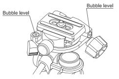
Adjust the level so that the bubble in inside of the marked circle.
