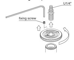
To change the U3/8" screw, loosen the fixing screw with an allen wrench (2.5mm width) and rotate the center column plate to remove from the center column.
