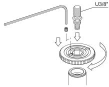
Flip the pan head attachment screw and put back to the center column plate.
