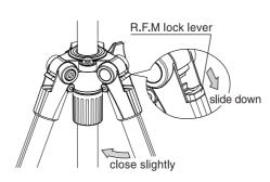
Close the leg slightly and slide the R.F.M lock lever
