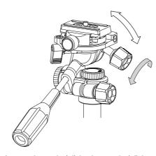
Loosen the vertical tilt knob or vertical tilt handle, and the level can be adjusted.
