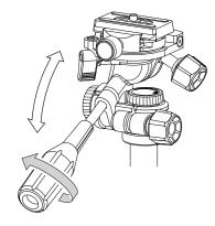
Loosen the pan & tilt handle, and the head will tilt back and forth.
