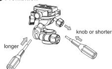
The longer pan handle should be installed to the rear of the head.
