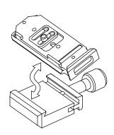
The bracket can be attached to an Arca-Type compatible tripod head.
