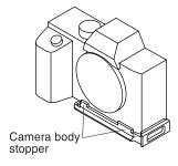
With the camera body stopper pressed against the front of the camera body, tighten the camera screw firmly.
