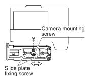
Loosen the slide plate fixing screws and adjust the position of the slide plate so that the camera mounting screw is in the position of the mounting screw hole of the camera.
