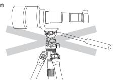
This product has been designed to handle equipment weighing under 4 kgs (8.81 lbs).
