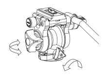
Loosen the pan lock knob, and the head will rotate horizontally.
