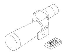
When your equipment has an anti-rotation pin mounting hole, match the locating pin to the hole and tighten the camera mounting screw.
