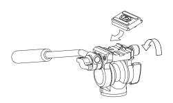
Fix the shoe lock knob firmly after inserting the quick release shoe to the platform. Please make sure the equipment is securely fixed to the pan head, before you use the pan
