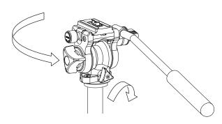
First, lock the pan lock knob, then grasp the pan handle and turn the head, counter-clockwise to loosen.
