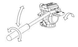
Loosen the pan handle lock knob to adjust the pan handle to the desired position.
