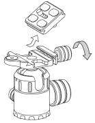
To remove the quick release shoe, loosen the shoe lock knob until the quick release shoe can be removed from the platform.
