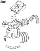
Fix the shoe lock knob firmly after inserting the quick release shoe onto the platform.
