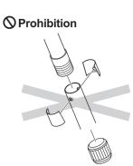
Do not remove the nut and take out pieces. If it has been removed, insert the pieces as per the above specification.
