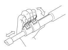
Flip up the leg lock lever to extend or shorten any of the individual leg sections to the desired length and press the leg lock lever flush against
