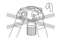
Please do not turn the center column stopper without a center column &/or an optional short center column. The internal parts may be damaged.
