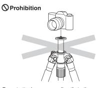
Do not attach a camera directly to the pan head
