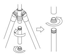
Remove the center column base stopper and then, remove the lower part
