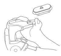
To remove the quick release shoe from the pan head, turn quick release lock lever and lift out platform from its back.
