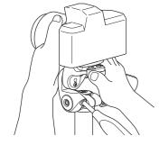
When attaching the camera to the pan head, check to make sure that the quick release shoe is engaged in the catch of the pan head before locking the lever.
