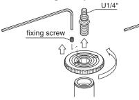
To change the U3/8" screw, loosen the fixing screw with an allen wrench (2.5mm width) and rotate the center column plate to remove from the center column. Then push out the panhead attachment screw from the bottom.
