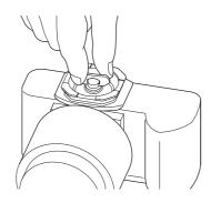
Align the length of the platform along the base of the camera body, and securely tighten the mounting wing nut.
