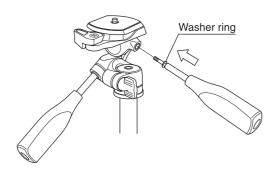
Check to see that there is a washer ring on the shaft of the vertical tilt handle, and then insert the shaft into the threaded hole located on the right side of the pan head. Screw handle all the way in until secure.
