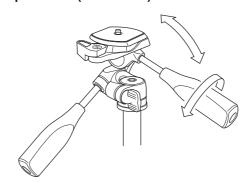
Loosen the Vertical tilt handle, and the level can be adjusted.
