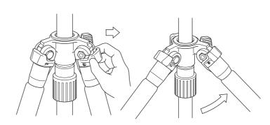
To change the angle of each leg, close the leg slightly, and then pull the leg angle adjustment lock out.
