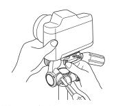
When you fix this quick release shoe to pan head, the quick release lock lever will return to the original position automatically.
