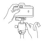
The camera platform can be locked into the position by the tightening the ball locking knob.
