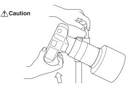
The camera call fall suddenly when the ball locking lever or locking lever is loosened, causing damages and injuries.
