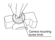
Insert the camera mounting screw (U 1/4") on the quick release plate in the place of the tripod attachment screw of your camera.
