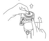
Remove the quick shoe by opening the locking lever and then pressing the release button.
