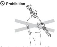
Carrying a tripod with a camera left on can result in unexpected accidents. We therefore, recommend you to remove your camera while carrying the tripod.
