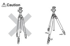
To prevent accidental equipment fall or tripod tipping over making sure all levers, knobs and handles on the tripod are securely tightened, and all three legs are opened all the way.
