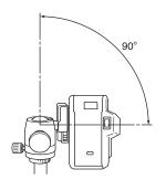
By using the vertical tilt collar, it will tilt down further to 90°.
