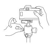
By turning the tension adjustment knob (located opposite of the ball locking knob), you can adjust the tension of the ball movement. Make sure to hold your camera while operating the tension adjustment knob. Make adjustments after loosening the locking knob slightly, so as to free the ball movement.
