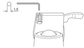
Over a long usage, the firmness of the locking lever may yield slightly. In such case, it is possible to make re-adjustments with the locking force adjustment knob.
