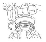
The body is moving freely when the lock ring is loosened.
