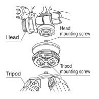
Make sure to attach tightly to the both of the head mounting screw and tripod mounting screw.
