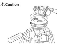
In case it is unable to be removed from a tripod, it can be removed to put a screw driver in the removing hollow.
