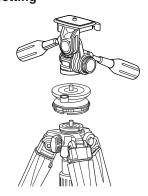
Mount the LEVELING UNIT 2 between a tripod and a tripod head.
