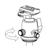
When the pan lock knob is loosened, the tripod head is rotated horizontally.
