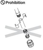
Do not remove the nut and take out pieces. If it has been removed, insert the pieces as per the above specification.
