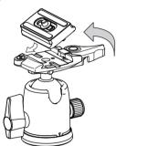
To reattach the shoe, slide it in from the shoe lock lever side.
