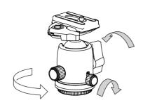
Tighten the ball lock lever and pan lock knob. Turn the head counter-clockwise to loosen.
