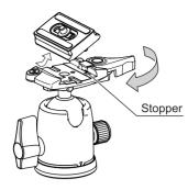
Remove the quick release shoe. Do not put the lock lever back by force as it has been stood by the stopper.
