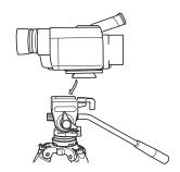
Attach the equipment onto the pan head and lock the shoe firmly with the shoe locking lever.
