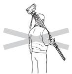
Carrying a tripod with equipment attached can result in unexpected accidents.
