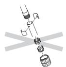
Do not remove the nut and take out pieces. If it has been removed, insert the pieces as per the above specification.
