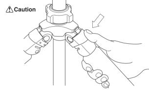
After choosing the desired leg angle, securely push in the adjustment lock.
