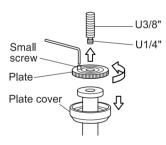
The pan head fixing screw is reversible for either large thread (U3/8") or small thread (U1/4").
