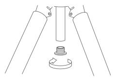
Remove the center column base stopper from the bottom of the center column.
