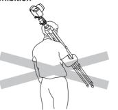
Carrying a tripod with a camera left on can result in unexpected accidents. We, therefore recommend you to remove your camera while you are carrying the tripod.
