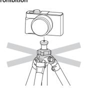
Do not attach camera directly to the threaded post of the center column. This may damage both of camera and tripod.
