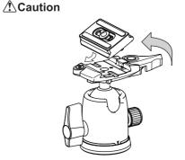
To reattach the shoe, slide it in from the shoe lock lever side.
