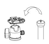
Always remove the pan head first before replacing the center column.
