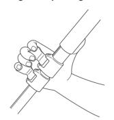
Flip up the leg lock lever to extend or shorten any of the individual leg sections to the desired length.
