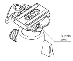
Adjust the bubble level to fit into center.
