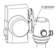
To set vertical camera position, place the platform into U-groove.
