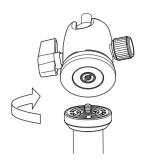
Set to the pan head attachment screw, and turn the head clockwise and fasten firmly.
