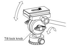
Loosen the tilt lock knob, and the head will tilt back and forth.
