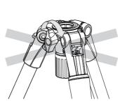
Please do not turn the center column stopper without a center column &/or an optional short center column. The internal parts may be damaged.
