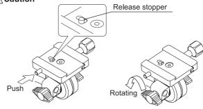
It is possible to intentionally disable the release stopper function by pressing and rotating the release lever.
