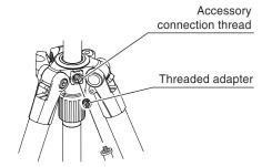
The tripod has 1/4" (if you take off the threaded adapter, 3/8") female thread which can be used to attach accessories, such as a light, a monitor, etc.
