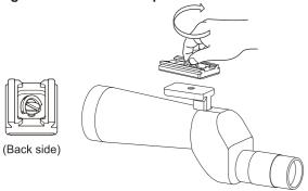
Attach the equipment screw hole and camera mounting screw and screwing lightly.
