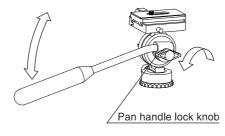
By loosen the pan handle lock knob, you can change the pan handle to the desired position. When adjusting the position of the pan handle, lock the tilt lock knob firmly.
