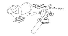
Press down the release button and insert the quick shoe into the camera platform.
