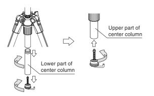
Remove the center column base stopper and then, remove the lower part of center column.
