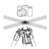
Do not attach camera directly to the threaded post of the center column. This may damage both camera and tripod.
