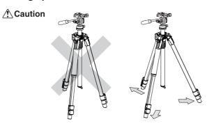
To prevent accidental equipment fall or tripod tipping over, making sure all levers, knobs and handles on the tripod are securely tightened, and all three legs are opened all the way.
