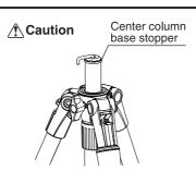
Insert the center column from the lower side of main body, and tighten the center column locking nut and the center column stopper. Make sure to re-attach the center column base stopper in order to prevent the center column falling out accidentally
