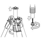
Loosen the center column locking nut and the center column stopper, and then pull out the center column.
