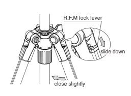
Close the leg slightly and slide the R.F.M lock lever down
