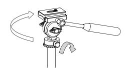
Set the pan head on the tripod's threaded post, and turn clockwise until it comes to a stop.
