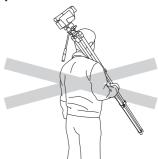
Carrying a tripod with a camera left on can result in unexpected accidents. We therefore, recommend you to remove your camera while carrying the
