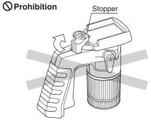
In this case, please do not put the quick release shoe locking lever back by force as it has been stood by the stopper.
