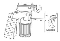
The camera platform rotates when the camera platform locking lever is loosened in the direction of the arrow.
