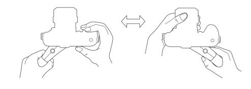
The position of the grip can be freely chosen as the camera platform rotates. Please fix the camera platform with the locking lever when you decide your required position.
