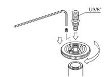
Flip the pan head attachment screw and put back to the center column plate. Screw in the center column plate and the pan head attachment screw. Tighten the fixing screw to avoid the rotating the center column plate while in use.
