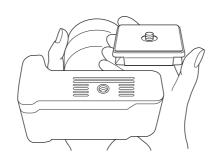
Insert the camera mounting screw of the quick release shoe in the place of the tripod attachment screw of your camera.
