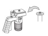
Remove the pan head when inverting
