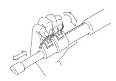
Flip up the leg lock lever to extend or shorten any of the individual leg sections to the desired length and press the leg lock lever flush against the leg to lock.
