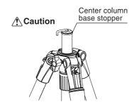
Insert the center column from the lower side of main body, and tighten the center column locking nut and the center column stopper.
