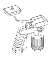
Attach the quick release shoe slide aslant from the quick release shoe locking lever. It will be closed automatically after attaching.
