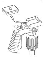
Remove the quick release shoe turning the quick release shoe locking lever.
