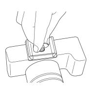
Turn the camera mounting screw knob and fix firmly.
