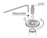
To change the U3/8" screw, loosen the fixing screw with an allen wrench (2.5mm width) and rotate the center column plate to remove from the center column. Then push out the pan head attachment screw from the bottom.
