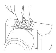
Align the length of the quick release shoe along the base of the camera body, and securely tighten the mounting wing nut.
