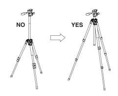
To avoid unnecessary camera vibrations, try to keep the center column height to a minimum.
