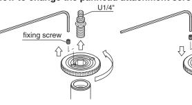
To change the U3/8" screw, loosen the fixing screw with an allen wrench (2.5mm width) and rotate the center column plate to remove from the center column. Then push out the panhead attachment screw from the bottom.
