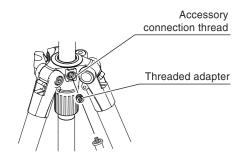
The tripod has 1/4" (if you take off the threaded adapter, 3/8") female thread which can be used to attach accessories, such as a light, a monitor, etc.
