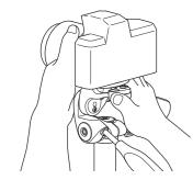
When attaching the camera to the pan head, check to make sure that the quick release shoe is engaged in the catch of the pan head before locking the lever.
