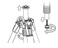
Remove the center column base stopper from the bottom of the center column.
