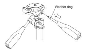
Remove the vertical tilt handle from the back of the pan & tilt handle where it is stored.
