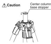
Insert the new replacement center column through the top, and tighten the locking collar.
