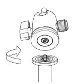
Set to the pan head attachment screw, and turn the head clockwise and fasten firmly.
