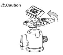
To reattach the shoe, slide it in from the shoe lock lever side.
