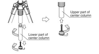
Remove the center column base stopper and then, remove the lower part
