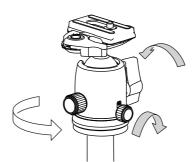
Tighten the ball lock lever and pan lock knob.
