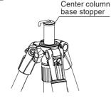
Insert the center column from the lower side of main body, and tighten the center column locking nut and the center column stopper.
