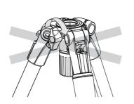
Please do not turn the center column stopper without a center column &/or an optional short center column. The internal parts may be damaged.
