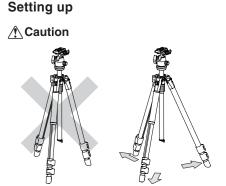
To prevent accidental equipment fall or tripod tipping over making sure all levers, knobs and handles on the tripod are securely tightened. And all of the three legs are opened all the way.
