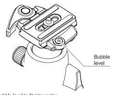
Adjust the bubble level to fit into center.
