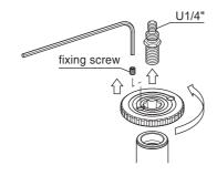
To change the U3/8" screw, loosen the fixing screw with an allen wrench (2.5mm width) and rotate the center column plate to remove from the center column. Then push put the pan head attachment screw from the bottom. Loosen the plate without removing the small screw.
