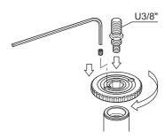
Flip the pan head attachment screw and put back to the center column plate. Screw in the center column plate and the pan head attachment screw. Tighten the fixing screw to avoid the rotating the center column plate while in use
