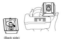
Screw the camera mounting screw on the tripod attachment screw of your camera and fix firmly.
