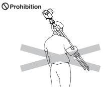
Carrying a tripod with a camera left on can result in unexpected accidents.
