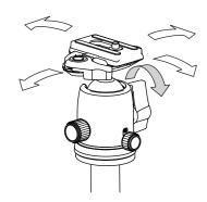
The platform can be moved freely while ball lock lever is loosened. Tighten the ball lock lever when a camera angle is determined.
