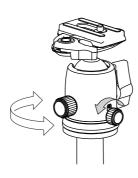
When the pan lock knob is loosened, the tripod head is rotated horizontally.
