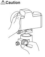
The platform can be moved freely while ball lock knob is loosened. Tighten the ball lock knob when a camera angle is determined.
