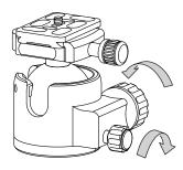
Tighten the ball lock knob and pan lock knob. When a tripod mounting screw is U3/8", remove a double screw adaptor.
