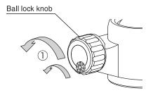
Friction adjustment provides an adequate amount of damping force for the ball movement, providing smooth camera movement and prevent sudden camera fall when loosening the ball lock knob.
