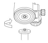
Fasten the ball lock knob and screw into a tripod mounting screw.
