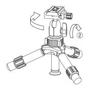
Set the new head, on the pan head attachment screw, and turn clockwise until it comes to a stop.
