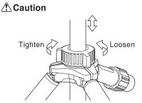
Hold onto the ball head with one hand, and loosen the center column locking collar with the other hand.
