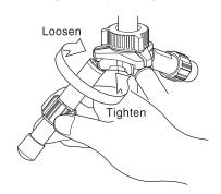
To extend any leg, turn the leg lock nut one helf turn counter-clockwise.
