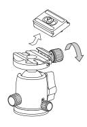
Remove the quick release shoe to loosen the shoe lock knob until the quick release shoe can be removed from the platform.
