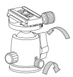
Tighten the ball lock lever and pan lock knob. When a pan head attachment screw of the tripod is U3/8", remove the double screw adaptor.
