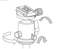
Tighten the ball lock lever and pan lock knob. Turn the head counter-clockwise to loosen.
