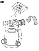
Fix the shoe lock knob firmly after inserting the quick release shoe to the platform. Please make sure the equipment is securely fixed to the ball head, before you use the ball head.
