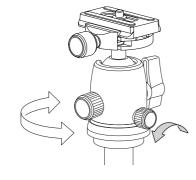
When the pan lock knob is loose, the head rotates horizontally.
