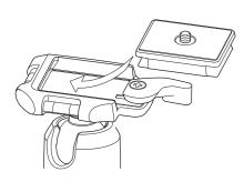
To reattach the shoe, slide it in from the shoe lock lever side. When it attaches, the shoe lock lever closes automatically.
