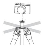
Do not attach camera directly to the threaded post of the center column.
