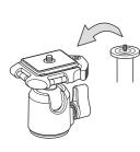
Remove the ball head when inverting or replacing the center column.
