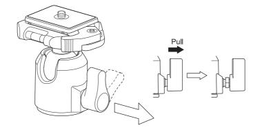
You can change a position of a ball lock knob. To change a position, turn the ball lock knob to your desired position when pulling a ball lock knob itself.
