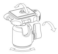
Camera platform and base plate will be rotated when the ball lock knob is
