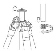
Remove the center column base stopper from the bottom of the center
