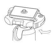
Push the shoe lock lever more to make sure the camera shoe is locked
