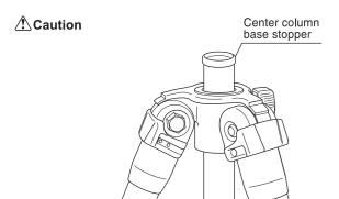
Insert the center column from the lower side of main body, and tighten the center column locking nut and the center column stopper. Make sure to re-attach the center column base stopper in order to prevent the center column falling out accidentally.
