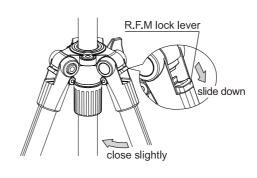
Close the leg slightly and slide the R.F.M lock lever down
