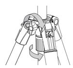
Tighten center column stopper and center column locking collar.
