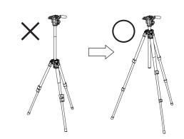
To avoid unnecessary camera vibrations, try to keep the center column height to a minimum.
