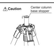
Insert the center column from the lower side of main body, and tighten the center column locking nut and the center column stopper. Make sure to re-attach the center column base stopper in order to prevent the center column falling out accidentally
