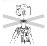
Do not attach camera directly to the pan head attachment screw of the center column. This may damage both camera and tripod.
