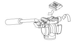
Fix the shoe lock knob firmly after inserting the quick release shoe to the platform. Please make sure the equipment is securely fixed to the pan head, before you use the pan head.
