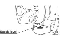
Adjust the level so that the bubble is inside of the marked circle.
