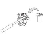
Remove the pan head when inverting
