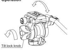
Loosen the tilt lock knob, and the head will tilt back and forth.
