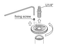
To change the U3/8" screw, loosen the fixing screw with an allen wrench (2.5mm width) and rotate the center column plate to remove from the center column. Then push out the pan head attachment screw from the
