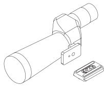
When your equipment has an anti-rotation pin mounting hole, match the locating pin to the hole and tighten the camera mounting screw.
