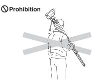
Carrying a tripod with a camera left on can result in unexpected accidents.
