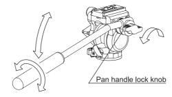
Loosen the pan handle lock knob to adjust the pan handle to the desired position.
