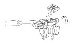
Remove the quick release shoe to loosen the shoe lock knob until the quick release shoe can be removed from the platform.
