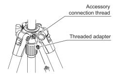
The tripod has 1/4" (if you take off the threaded adapter, 3/8") female thread which can be used to attach accessories, such as a light, a monitor, etc.
