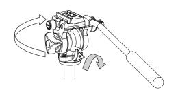
Set the pan head on the tripod's threaded post, and turn clockwise until it comes to a stop. Tighten the pan lock knob and turn clockwise slightly more.
