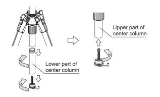
Remove the center column base stopper and then, remove the lower part of center column.
