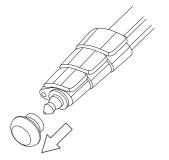
If you pull out the rubber feet in the direction of the arrow, it becomes a spike, so you can use it depending on where you use the tripod. Remove any dirt before attaching the rubber feet.
