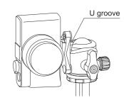
To set vertical camera position. place the platoform into U-Gloove.
