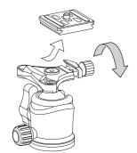
To remove the quick release shoe, loosen the shoe lock knob until the quick release shoe can be removed from the platform.
