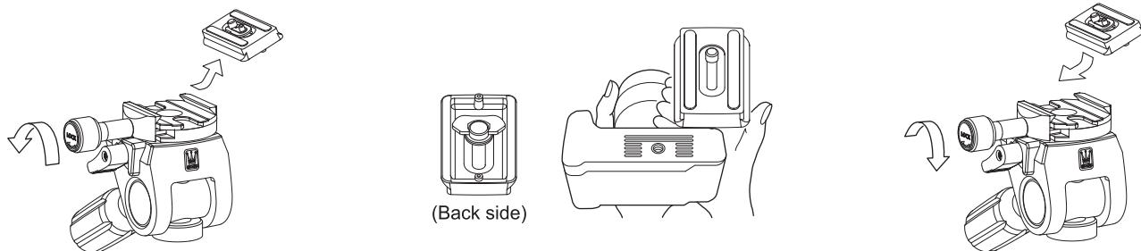
To remove the quick release shoe, loosen the shoe lock knob until the quick release shoe can be removed from the platform.
