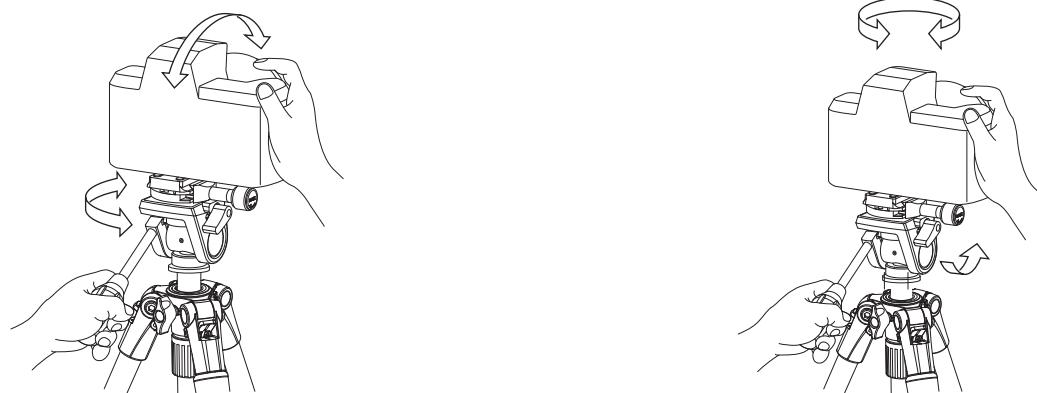
When you unlock the handle, your camera is free to move up and down. When the pan & tilt handle is unlocked, you can pan & tilt simultaneously.
