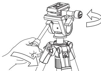
With your hands off the trigger, turn the head forcefully counterclockwise to loosen the head. Squeeze the grip & trigger and turn the head counterclockwise to remove the head.
