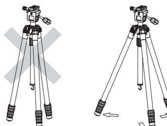
To prevent accidental equipment fall or tripod tipping over, make sure all levers, knobs and handles on the tripod are securely tightened. And all of the three legs are opened all the way.
